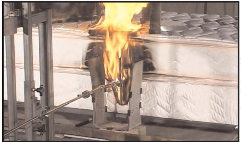
A dual propane burner is used in the CPSC test rig to simulate how burning bedclothes (heat flux and duration) may affect a mattress and box spring or a mattress alone.
