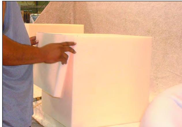
In bonding foam to foam, the objective is to create a joint where the foam will tear before the bond separates.
