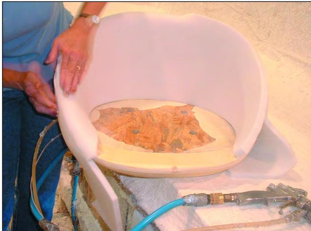
Special adhesives are available for applying foam to composite plastics.
