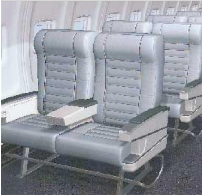
While GIF foam seating promises the possibility of eliminating the need for fireblock fabrics, there are tradeoffs. When the fireblock is removed, comprehensive composite flammability testing will be required on each new seat design. Total fabricated seat weight may also change.
