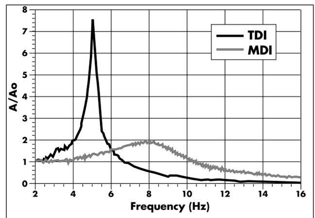
**An ARCO Chemical study presented at SAE (February 1996) indicates that TDI foam is effective at dampening vibration waves at typical highway speeds.**
