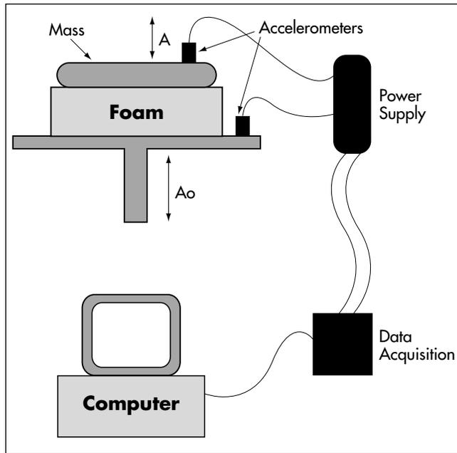
**ACDF testing uses accelerometers to gather vibrational wave data from the source as well as through different foams to document transmissivity rates over real time.**
