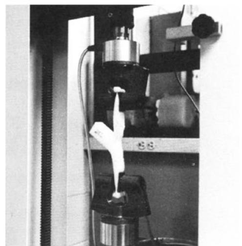
▲ *Tests for tear strength analyze both long term durability and the foam’s ability to be handled during product assembly.*
