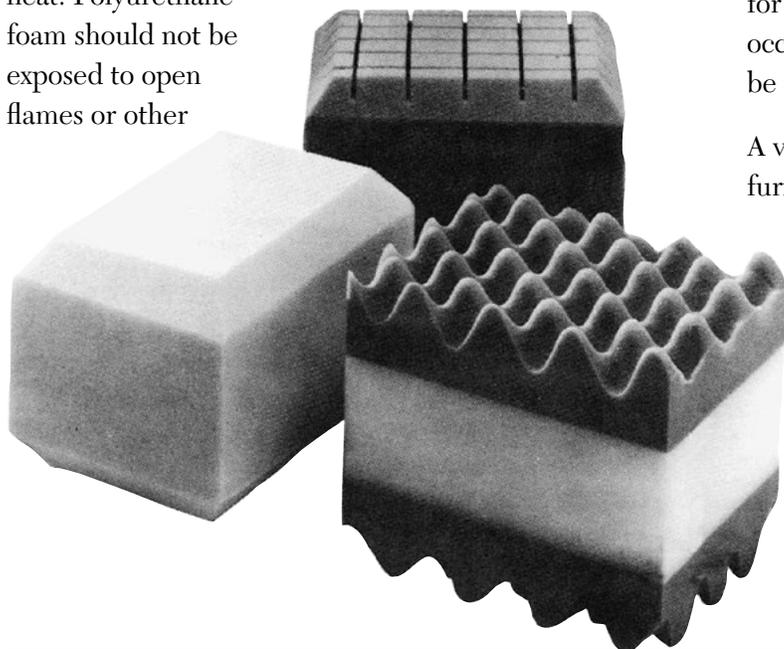
Air flow through foam should be a minimum of 2.0 cfm.
