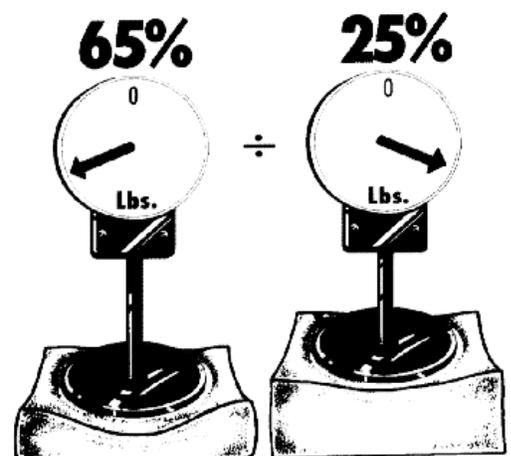
When specifying compression modulus, it's also important to understand the relationship it has to foam firmness, especially when considering the **ratio** of seat to back firmness. A rule of thumb is that the more weight placed on the back cushion, the less difference there can be between the firmness of the seat and back cushion. The same holds true for compression modulus. The support capabilities of the back cushion should complement the seat cushion.
