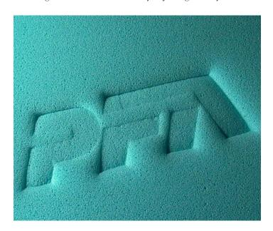
Viscoelastic (memory) foam is characterized by slow recovery after compression. Its ability to closely contour to shapes allows surface pressure to be distributed over a wide area.
