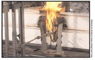
A dual propane burner is used in the CPSC test rig to simulate how burning bedclothes (heat flux and duration) may affect a mattress and box spring or a mattress alone.
