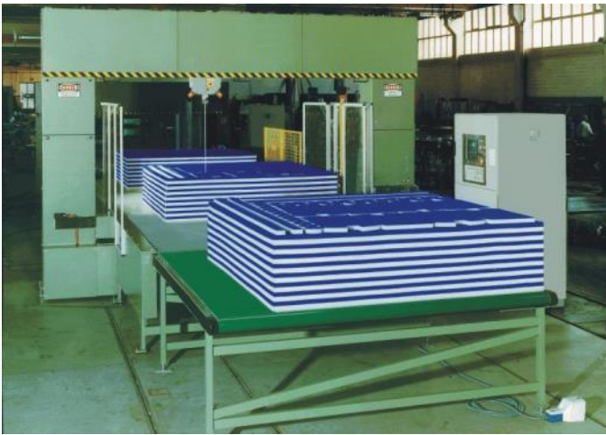
CAD-CNC vertical saws are able to cut buns or sheets and a variety of materials such as FPF, bonded foam and fiber.
