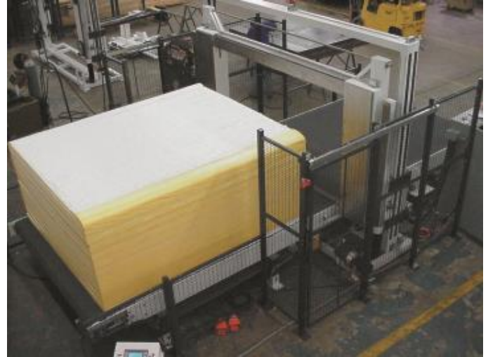
Horizontal slitters allow fabricators to reduce large FPF blocks to sheets for applications such as mattress toppers.
