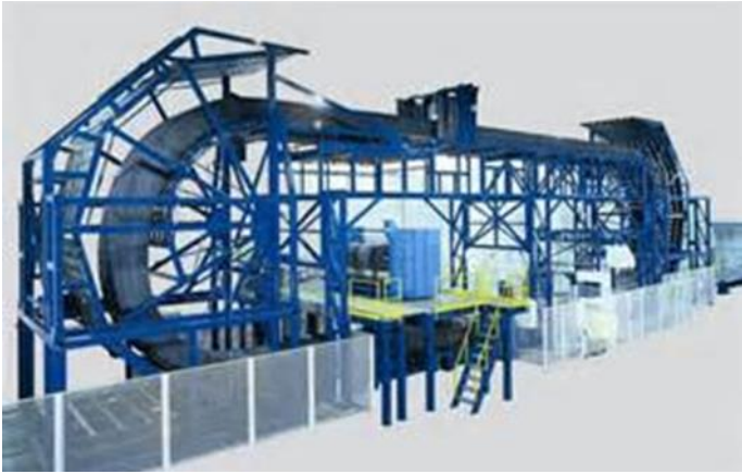
Loopers speed up the process of splitting long blocks of foam.
