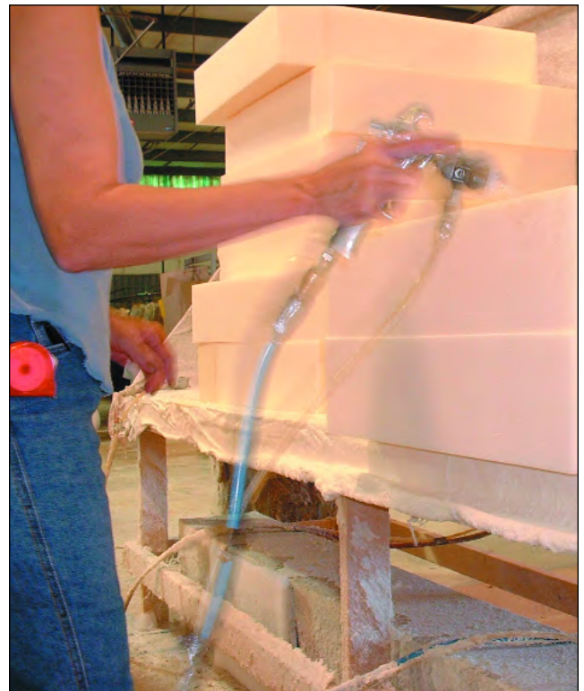
Many FPF fabrications require the use of adhesives to bond foam to foam, foam to fiber, or foam to non-porous surfaces such as plastic, metal or wood.
