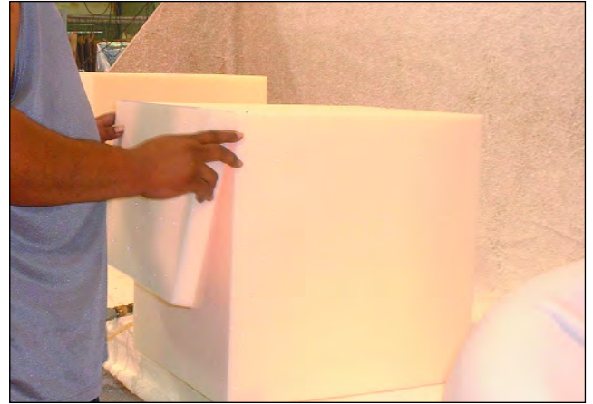
In bonding foam to foam, the objective is to create a joint where the foam will tear before the bond separates.
