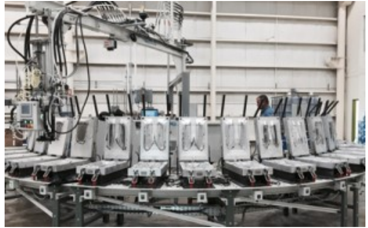
A carousel of molds for making foam components.
