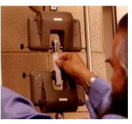
**Tensile strength and elongation** are related. Tensile is the stress required to pull the foam apart. As the foam is being pulled, elongation is a measure of how much the foam stretches before it comes apart.
